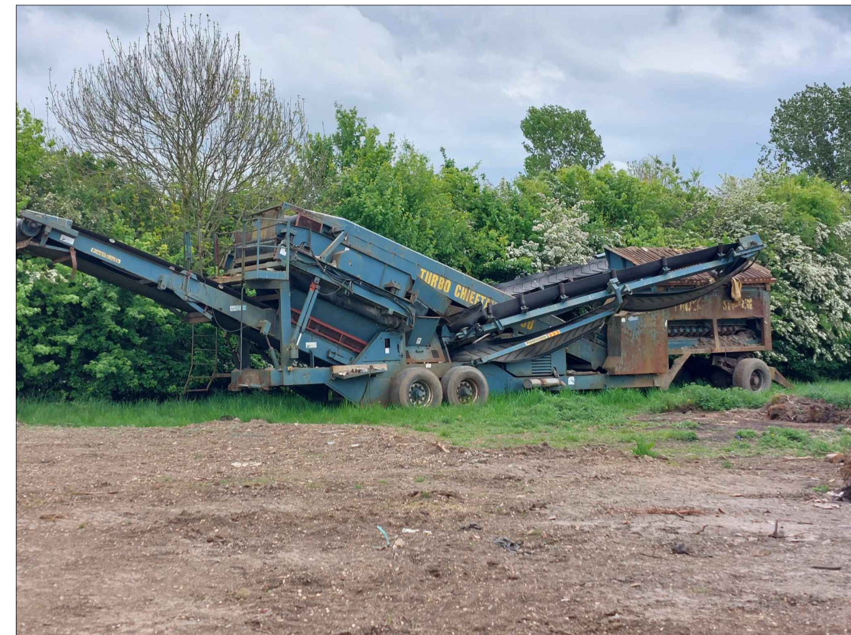
TYPICAL TOPSOIL SCREENER
